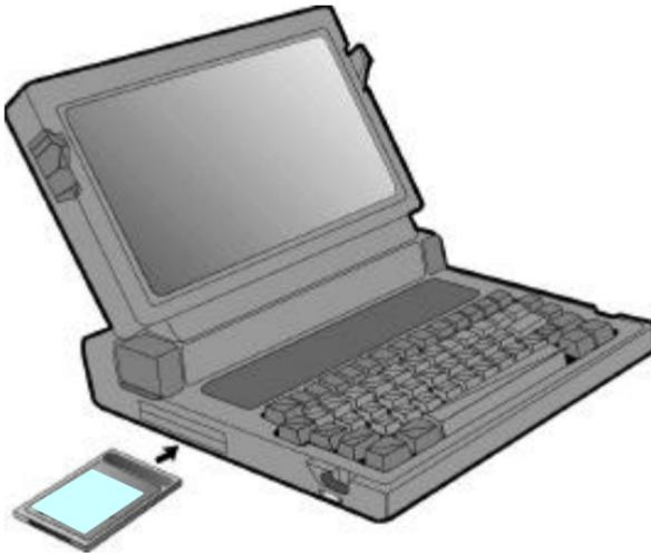
**Figure 2-3.1 Insert the ENW-3502-FC into the Socket**
