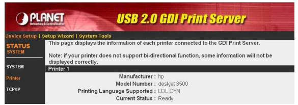
This page lists the information and the status of the printer connected to the GDI Print Server USB port. The printer information includes manufacturer, model number and the supported printing language. The status of the printer include "Ready", "Off Line" or "Paper Out".
