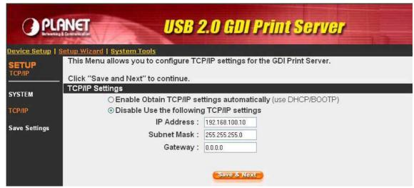
You can configure the GDI Print Server to automatically get IP from DHCP server or manually specify static IP.
