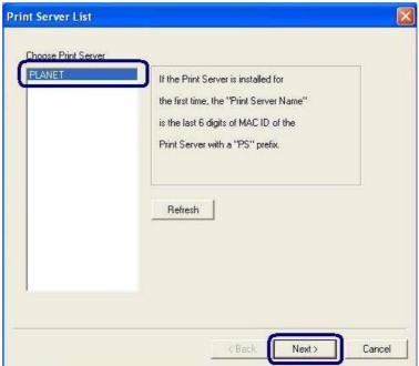
NOTE: If this is the first time you configure the print server, the "Print Server Name" will the same as the "Device Name" printed at the bottom of the print server.
