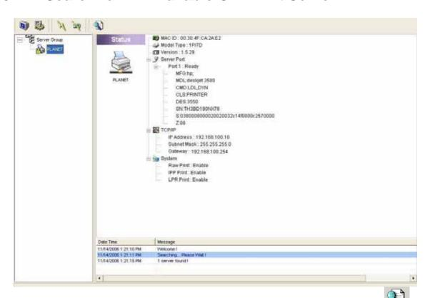
Every time when you run the "Server Manager" configuration utility, click the "Search" icon the tool bar. The configuration utility will delay for several seconds because the utility is using system's available network protocols to search for all GDI Print Servers on the network. All available GDI Print Servers will be listed under "Server Group" on the left side of the window.
