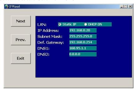
**LAN:** You can configure this ICA-108/108W to obtain its address automatically or manually assign. If there is a DHCP server in your network environment and you select "**DHCP ON**", ICA-108/108W can automatically obtain an IP address. If you don't have DHCP server or you want to use fixed IP address, please select "**Static IP**" and fill in the following fields with proper parameters.
