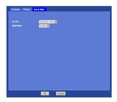
**IR LEDs:** User can turn on, off or scheduling the built-in IR LEDs. This function is very useful under low illumination environment even 0 Lux. Note that CMOS sensor will turn to black and white mode while IR LEDs turning on.
