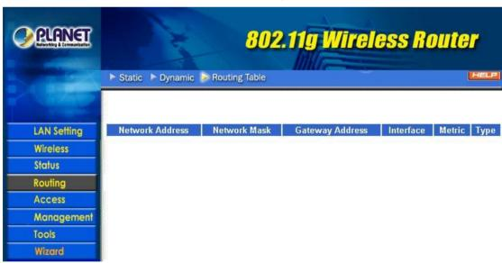
**Network Address:** Displays the network IP address of the connected node. **Network Mask:** Displays the network (subnet) mask of the connected node. **Gateway Address:** Displays the gateway address of the connected node. **Interface:** Displays whether the node is connected via a WAN or LAN.
