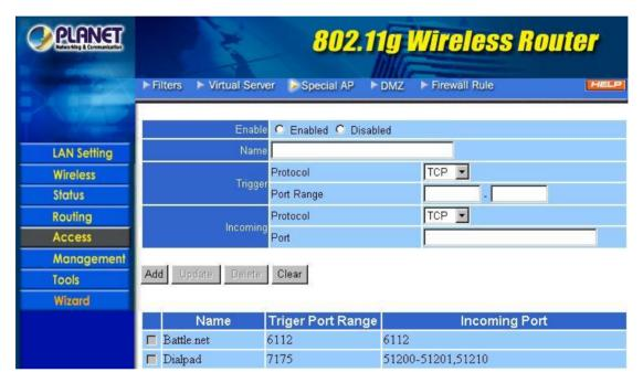
**Enable:** Click to enable or disable the application profile. When enabled, users will be able to connect to the application via the WRT-410 WAN connection. Click Disabled on a profile to prevent users from accessing the application on the WAN.
