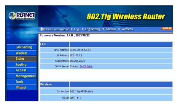
**Firmware Version:** Displays the latest build of the WRT-410 firmware interface. After upgrading the firmware in Tools -> Firmware, check this to ensure that your firmware was successfully upgraded.
