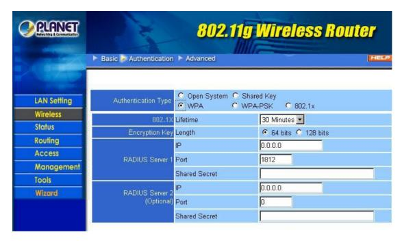
**Lifetime:** Select proper time interval from the drop-down list. Once the lifetime expires, the Encryption key will be renewed by RADIUS server automatically.
