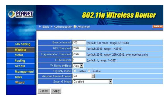
**Beacon Interval:** Type the beacon interval in the field. You can specify a value from 20 to 1000. The default beacon interval is 100.
