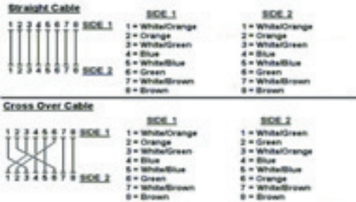
Figure A-1: Straight-Through and Crossover Cable
