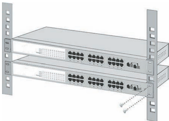
Figure 2-5 Mounting the Switch in a Rack
