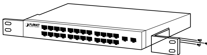
Figure 4: Attaching the brackets to the FGSW-2402S
