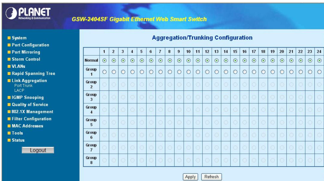
Figure 4-29 Aggregation/Trunking Configuration screen
