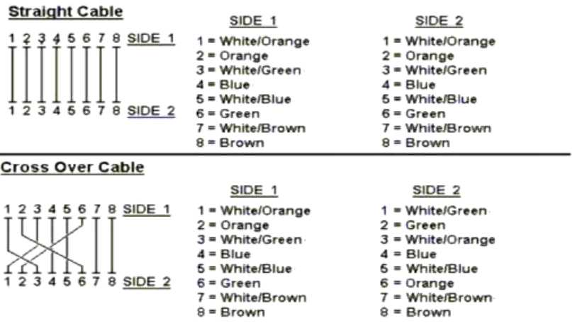
Figure A-1: Straight-Through and Crossover Cable
