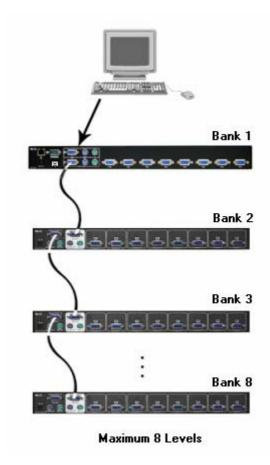
Connect Keyboard, Mouse and Monitor to the console port (Local console block) of IKVM-8000.
