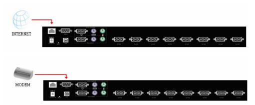
The rear side of IKVM-8000 provides a RJ-45 connector for Ethernet. The connector is used either for a 100Mbps 100BASE-TX connection or for a 10Mbps 10BASE-T connection. The adapter can sense the connection speed and will adjust to the appropriate operation mode automatically.
