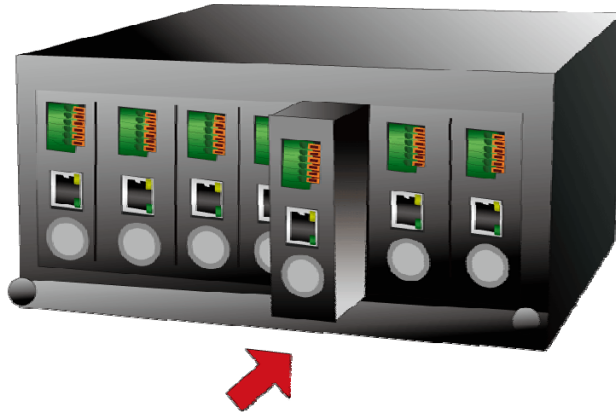
Figure 2-1: Insert a media converter into an available slot
