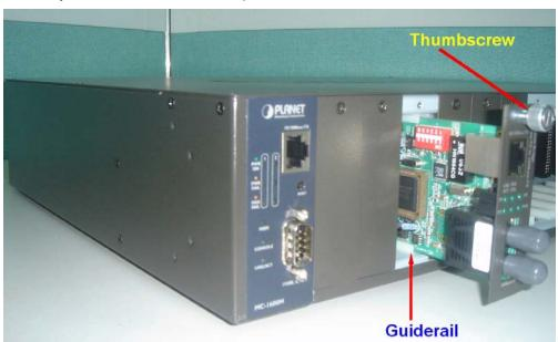
Step 4: Secure the FST-80x /GST-70x Media Converter board to the chassis by tightening the thumbscrew.
