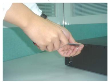
Step 3: Slide the FST-80x /GST-70x Media Converter board into the expansion slot, aligning it with the guide rails, until it firmly connects to the chassis' backplane.
