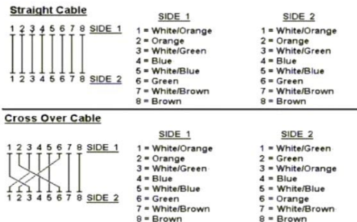
Figure A-1: Straight-Through and Crossover Cable
