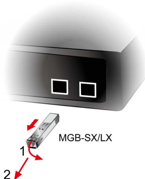
Figure 2-17: How to Pull Out the SFP/SFP+ Transceiver
