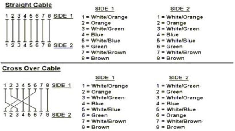
Figure A-1: Straight-Through and Crossover Cable
