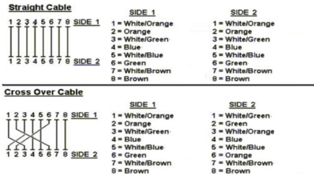
Figure A-1 Straight-Through and Crossover Cable
