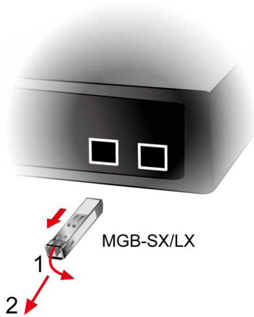
Figure 2-17: How to Pull Out the SFP/SFP+ Transceiver
