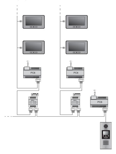
4.3 Gateway Mode: : In this mode, the first door station can call all the monitors and can connect 7 BDUs at most.
