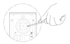
Use a screwdriver to loosen the screw and then adjust the angle of the camera ,then fix the screw.
