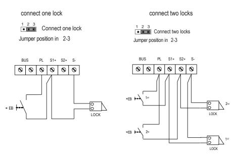
Door Lock Controlled with Dry Contact
