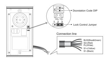
Lock Control Jumper: To select the lock type.
