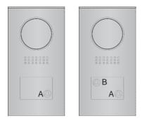
Note:Monitors response button A must set the user code from 0 to 15.and button B set the user code from 16 to 31.
