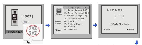
Press "#",Input "8002", then input Setup Code or Admin Code
