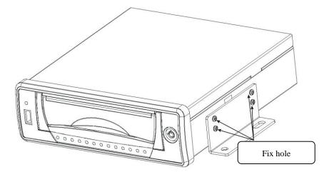
3. Place the rubber pad under the installation bracket.
