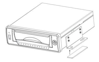
$4_{\text{S}}$  Fix the device in the specified position.
