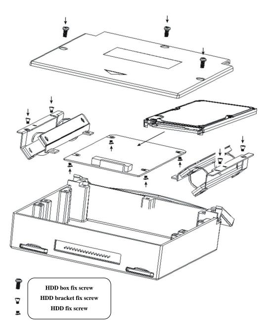
3) After completing HDD, insert it into device HDD slot and then lock.
