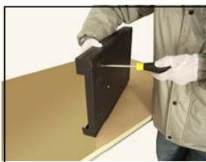
④fix the screw of hard disk
