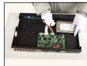
⑥connect the power wire
