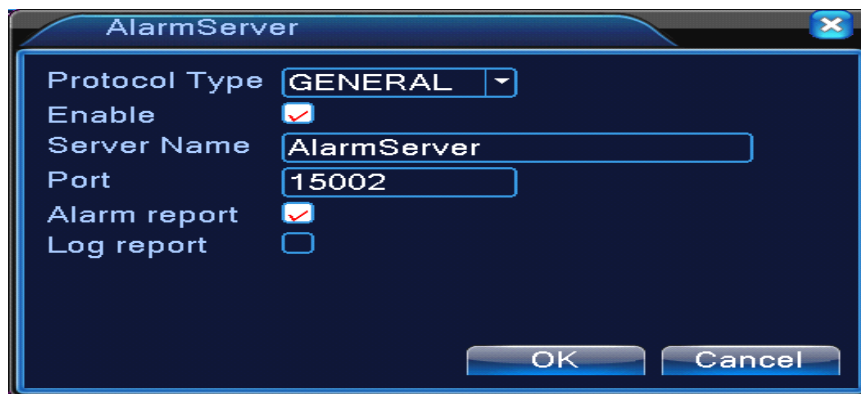
Pic: 4.30 alarm server setting
