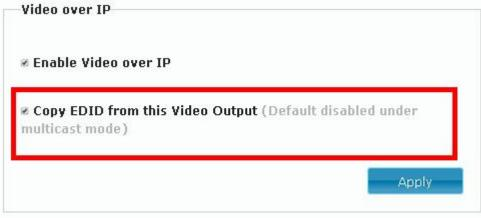
R Video over IP: This function setup the video signals send from network, select Copy EDID from this Video Output and enter "Apply" finish setting (pick up this item will auto copy R TV EDID)
