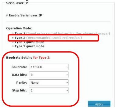
Serial over IP: This function setup Serial (RS232) signal sends from network
