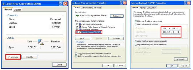
(IP address: 169.254.111.111 Submask: 255.255.0.0 Getway and DNS are not required)
