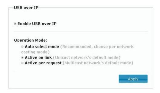
USB over IP Setup: This function setup the USB signals send from network.
