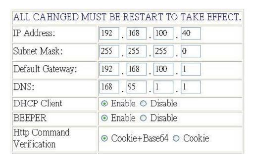
Click the "Setup" button on the left side; fill in the proper IP address, Subnet Mask, Default Gateway, DNS. If you choose to use DHCP, please make sure that your network support DHCP service so the XL-IPM4014 will search and gain an IP address automatically when it starts. You can also control the Beeper sound.
