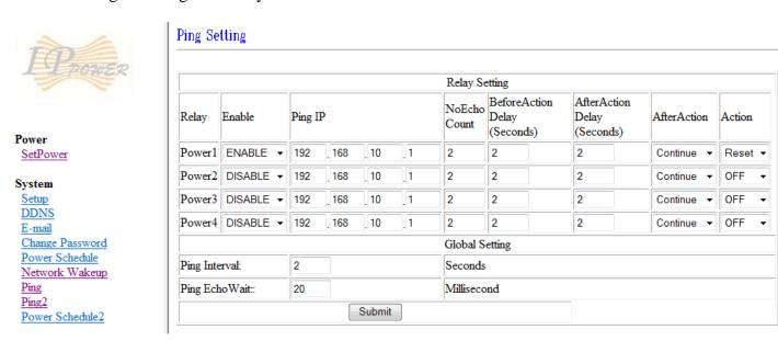
For every power outlet you can set default action if there is no response on ping. U can also set "Before Action Delay" and "After action Delay" when ping function should be restored.
