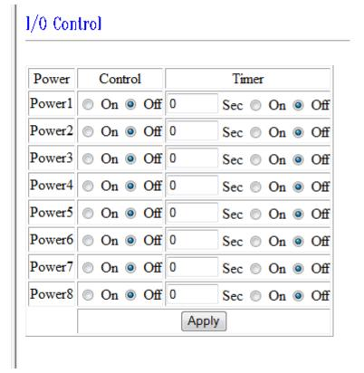
XL-IPM4014 can control 8 outputs individually at the same time. User can choose power on or power off with an electrical outlet. User may fill in the corresponding columns with the delay time you wish in seconds, then choose the action after delay to be on or off.
