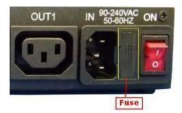
2.) Carefully remove the fuse holder with a flat screwdriver.
