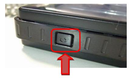
Step 3 : Press One time ( short) the "Reset button" of IPM-401W and then there is one long beep which means the WPS function of IPM-401W enable.
