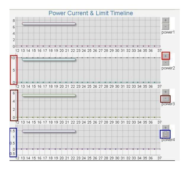
B-3 User can change the time gap difference by mouse : Select the time area you would like show on chart . To go back to original display as 10 seconds , please click "Current Limit" of IO Control section at left area .
