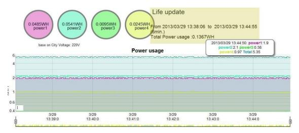
A. There are 4 color coding round signs on the left side show the total WH (Watt –Hour) of each power consumption in select area. User can move the 2 time gap sign to get the total consumed WH value of the select time range.
