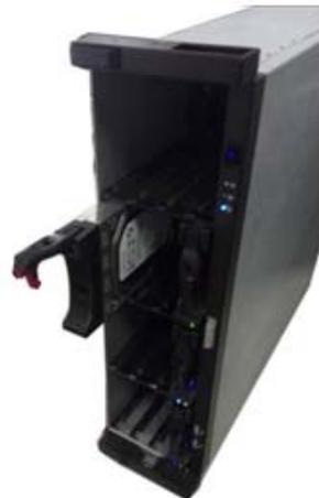
② Put the HDD to the HDD box at the front panel of the device. .
