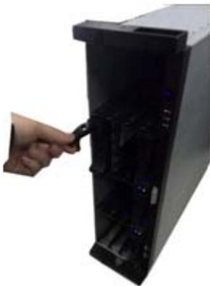
③ Please pull the handle up when you are inputing the HDD box in case the the handle collides with the front panel
