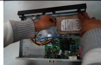
6. Connect the HDD cable and power cable.
