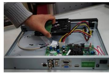
3. Place the HDD in accordance with the four holes in the bottom.
