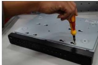
5. Fix the HDD firmly.
