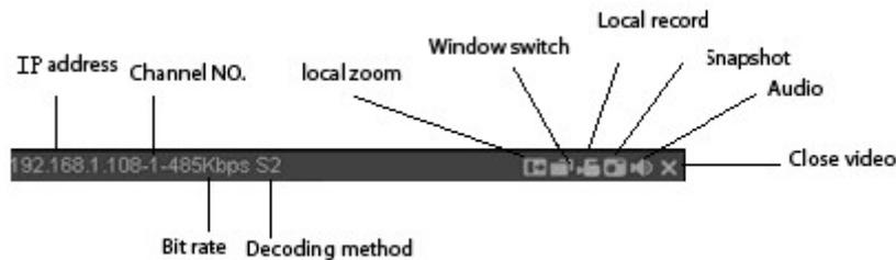
Figure 7-7 Real-time Monitor
