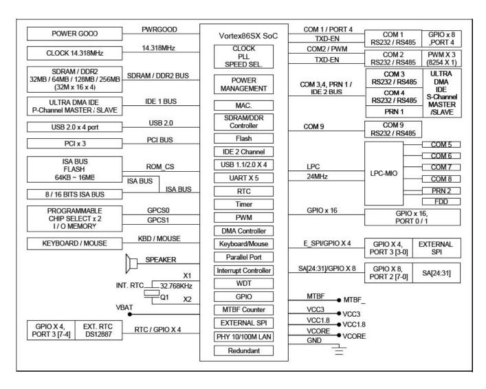
GPIO port 0,1 and 2 are always free for use normally. If your system does not use external RTC and SPI, GPIO port 3 is also free for use. Developer also can disable COM1 to select GPIO port 4. The actual free GPIO pins depend on your system. Please check it before using GPIO.
