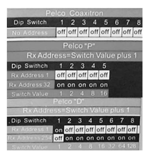
With reference to the above chart: When all code switches are under 'OFF'' status on speed dome, address code is 1. When you input Numerical key No.1 on control keyboard, then press CAM key for confirmation showing that set keyboard address as No.1 control address., At this time, keyboard can control speed dome camera(its control address is 0001). Other address is to be set as above.
