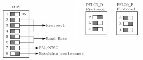
The 2st, 3nd and 4rd bits in FUN are used to set communication protocol (see following figure)
