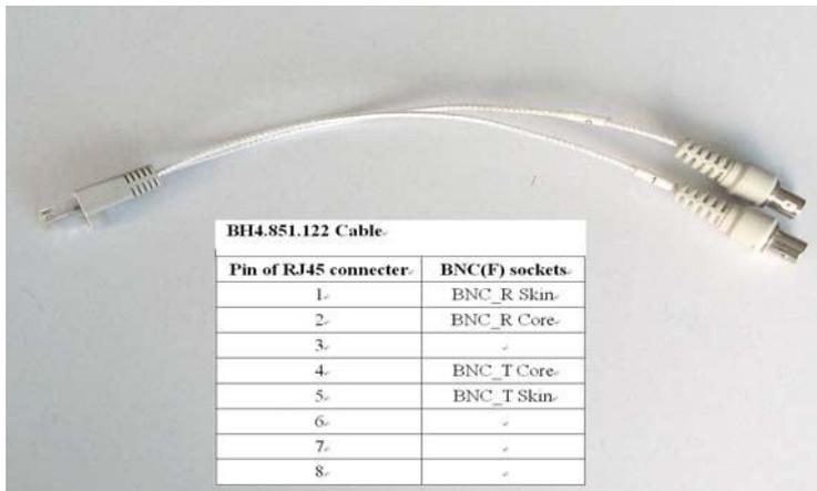
Fig. 3.1-2 75Ω converting cable
