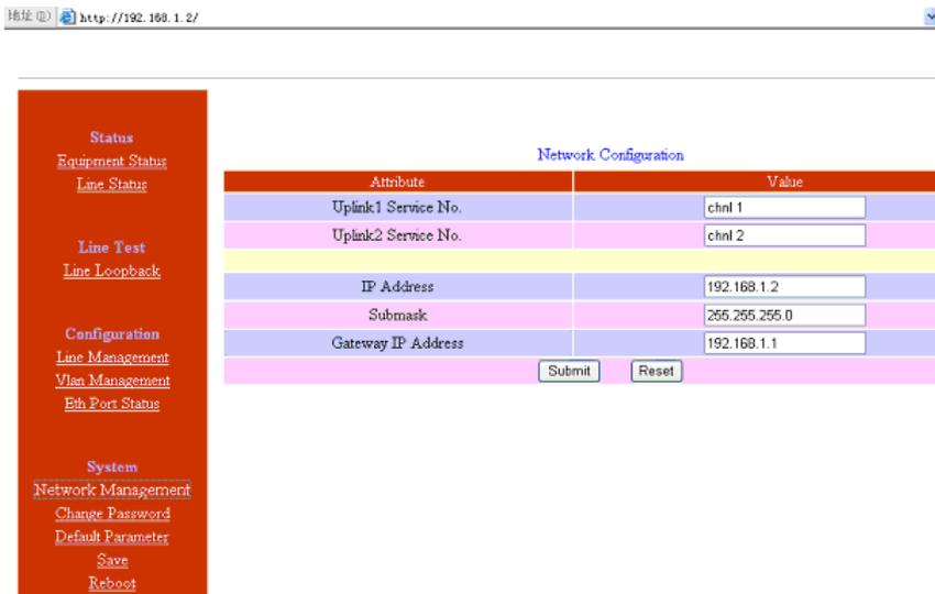
Fig 5.4-1 network configuration system
