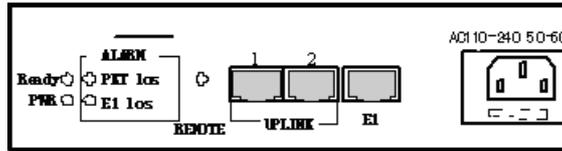
Fig. 2.3.1 E1 over Ethernet Multiplexer (220V AC)
