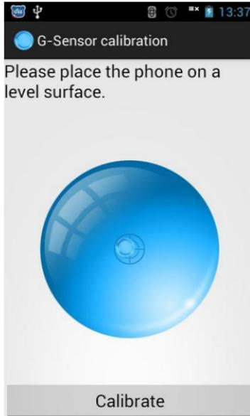
Click “Calibrate” to start this program. When the water ball is located in the cross center, the calibration has finished and press “ok” to accomplish the calibration.
