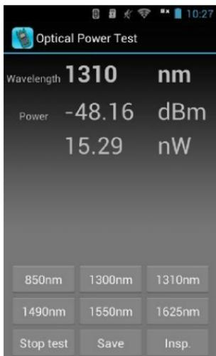
There are six wavelengths as calibration wavelength, choose corresponding wavelength can test current optical power value. It is shown as dBm and xW when having a test. User can stop testing by pressing "Stop Test", and the data displayed is the latest testing result. You can also choose save current test result, in help of checking afterwards. As following:
