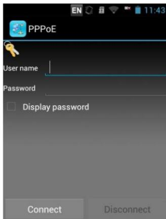
Input the user name and password, click connect to do the PPPoE dial, the equipment will memorize the user name and password automatically. User can test the web browsing.
