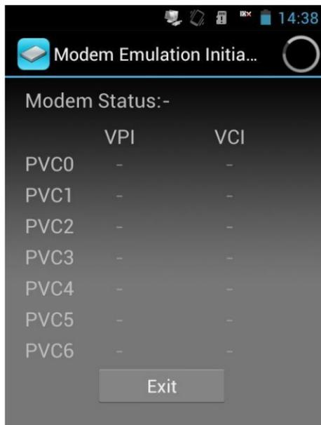
The tester will emulate user Modem to realize PPPoE dial through PC. (If the VPI/VCI value needs to be modified, please modify it from Modem Parameter window). Tester can realize PPPoE dial through user Modem emulation, and check the fault of user Modem. If it needs to exit Modem Emulation state, please Click **Exit!** to exit it.
