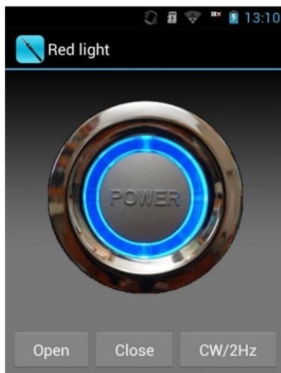
Click "Open" to turn on the VFL, and click "Close" to turn off the VFL. CW/2Hz is the switch button of the continuous and modulated light, the tester can memorize the VFL mode automatically.
