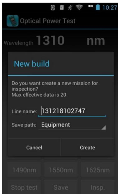
Input the name of the line to separate different lines. Inspection significance is: test one fiber on different positions of the optical power value, then draw the power curve (test curve is similar to the OTDR), you can view any attenuation values between 2 points.
