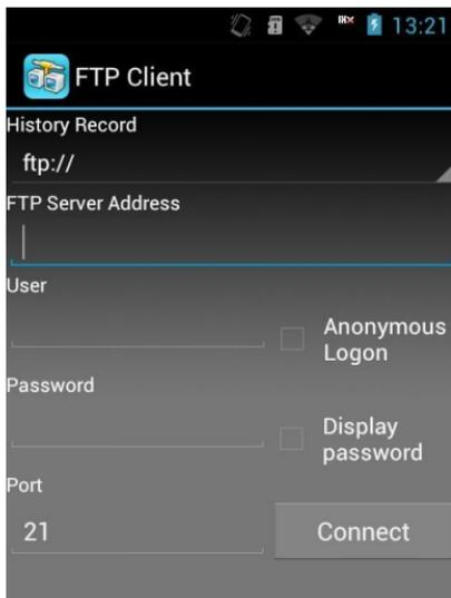
Typed FTP server address, user name, password and port number, and then clicking "Connect" can log on FTP server. The system will memorize the logged on FTP server address, user name, password and port number.
