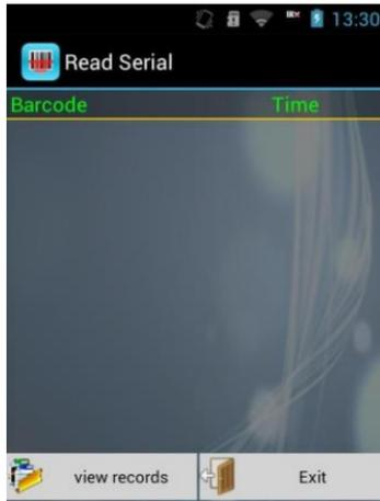
In the "Read Serial" interface, after pressing "SCAN" key on the side, it can work. The red light just aim at bar code, the test result will show on screen. Tester can scan continuously and show the scan result in table, and record the scan time. A prompt box about whether store will be pop up when exit.
