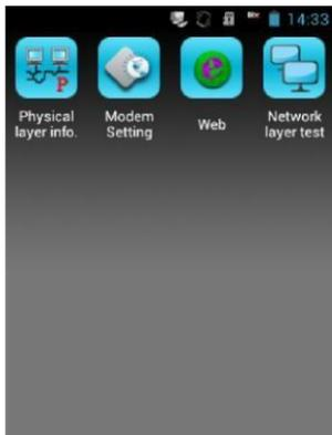
Physical layer test can test physical layer parameter, which including xDSL connection status, connection mode, Upstream/downstream channel rate, noise margin, attenuation, the output power, the number of error codes (CRC, HEC, FEC, NCD, OCD) and channel bits picture.
