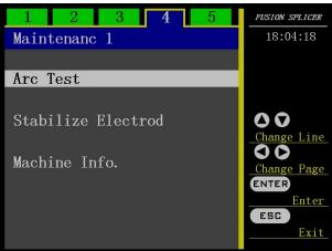
Press " $\blacktriangle$ " " $\blacktriangledown$ " to move the cursor, press "ENTER" to enter the program that you desire to get into, press " $\blacktriangle$ " " $\blacktriangledown$ " over again to modify the parameter values(via moving the cursor in the small pane); and press the key "ENTER" to confirm, so that the modification has completed. Then, press "ESC" to quit.
