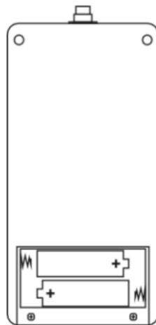
2. Installing the battery
