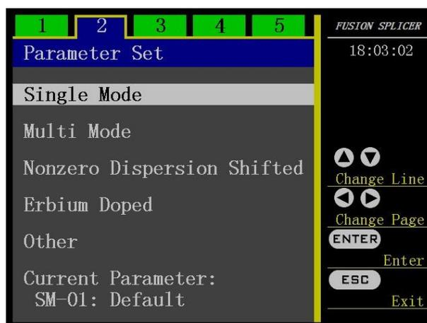
Press "▲" "▼" to move the cursor, and press "F1" to enter the "Fusion Splicing Mode" program that you want to get into.
