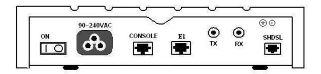
The rear panel of this model is including power switch, power socket, RJ-45 console, RJ-45 G.703, BNC jack for transmitting and receiving and RJ-45 for SHDSL from left to right.
