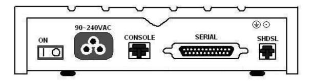
The rear panel of this model is including power switch, power socket, RJ-45 for console cable, DB-25(Female) for V.35 cable and RJ-45 for SHDSL from left to right.
