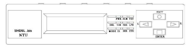
Front panel can be separated into three parts: LCD display, LED indicator and Keypads.
