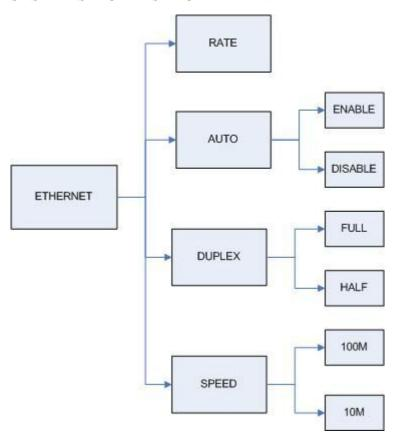
If you set Ethernet Auto Negotiation is **Enable**, the default setting on **Duplex** is Full and **Speed** is 100M.
