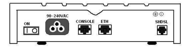
The rear panel of this model is including power switch, power socket, RJ-45 for console cable, LAN for Ethernet cable and RJ-45 for SHDSL from left to right.
