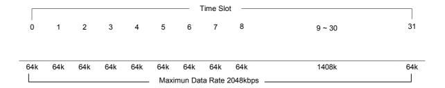
ITU 991.2 (2004) (G.SHDSL .Bis) supports data rate up to 56964Kbps, but G.703 (E1) only supports data rate of 2048kbps so the maximum data rate of SHDSL line, connected with E1
