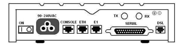
The rear panel of this model is including power switch, power socket, RJ-45 for console cable, LAN for Ethernet cable, RJ-45 G.703, BNC jack for transmitting and receiving, DB-25(Female) for V.35 cable and RJ-45 for SHDSL from left to right.
