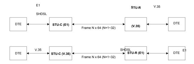
Time slot, N value, is place of data in the frame. Time Slot Number 1~31 (N=1~31) is Fractional E1 and Time Slot Number 32 (N=32) is unframed.
