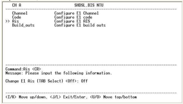
AIS (Alarm Indication Signal) is a method to inform the remote connection that there is a signal or sync problem with the E1. AIS is only valid in framed mode E1, not in Unframed E1. The setting here of AIS enabled (on) or not (off) and is for testing with AIS. When enabled, the E1 will transmit the AIS and it should be confirmed at the remote device (AIS indication lit). After testing, please turn AIS back off.
