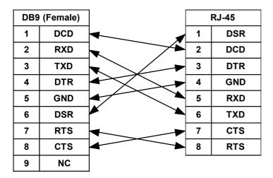
The table below displays Serial Interface Pin Assignments for the DCE Mode.
