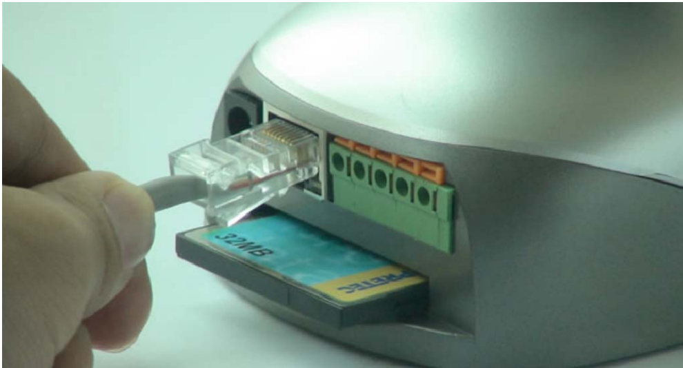
Figure 11 Connecting the Ethernet wire
