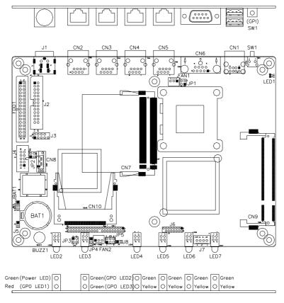
Jumpers on IB798PageJBAT1: Clear CMOS Setting9JP4: CF Card Master / Slave Selection9JP3: HDD UDMA Selection9
