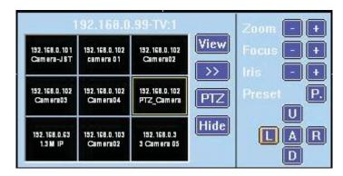
PTZ can only be controled when PTZ camera is selected. It's nearly the same with the operations on PTZ control panel. But you can only call the preset you have set. You can't set the preset here.
