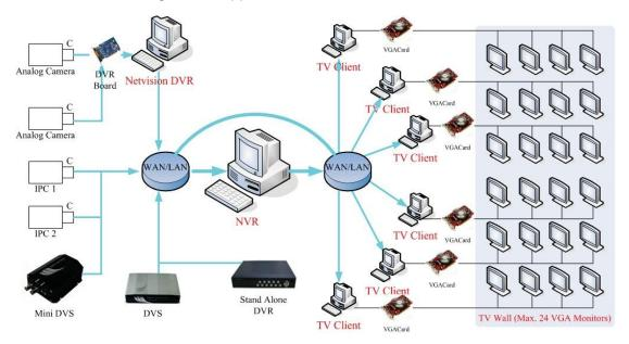
The frame diagram of application is as below:
