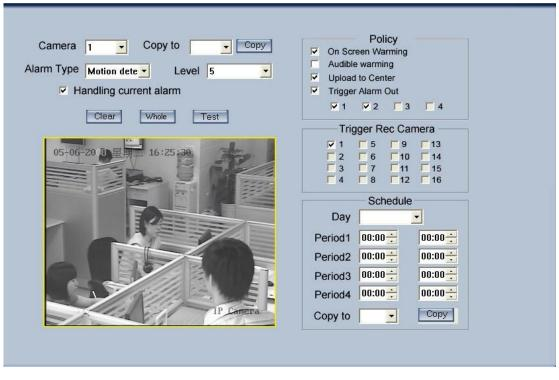
**[Camera]** Select a camera to be set from the drop-down list and you can copy the configuration to the other cameras by clicking copy button.
