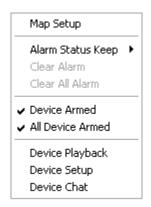
Click **Device Armed /All Devices Armed** (for more than one devices) to select alarm setup. Then, the device, including its cameras and sensors will turn golden yellow. When a camera detects a motion alarm, it will turn red and blink. At the same time, the video of the camera will be displayed automatically on the left screen if the setup in the server is suitable.
