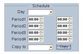
**Copy to** After finishing one channel, if you want to set any other channels' configuration as the same as this camera, you can select channel number from drop-down list, and press button.
