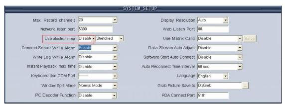
After you enable this function, videos of corresponding cameras will be displayed on the left screen when alarms are triggered out. Of course, you should confirm your setup in the device is suitable first.
