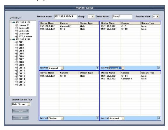
The only thing you have to do is setting the interval. You can set it as 5, 10, 15 and 20 seconds etc. The greatest interval here you can set is 60 seconds.
