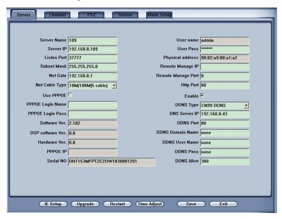
For DG Series EM-DVR, the interfaces are not exactly the same as DH Series. Remote setup for DG Series EM-DVR includes Server, Channel, Record, PTZ, Sensor, Alarm and User.
