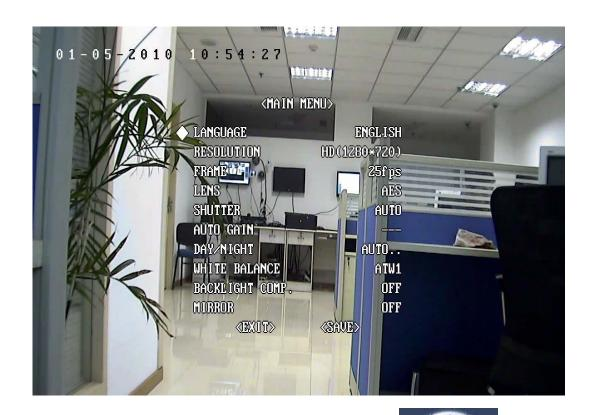
When you enter the menu, you can control it by using up, down, left and right buttons. Press IRIS – (IRIS – (I
