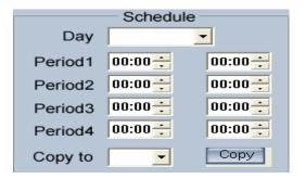
**Copy to** After finishing one channel, if you want to set any other channels' configuration as the same as this camera, you can select channel number from drop-down list, and press Copy button.
