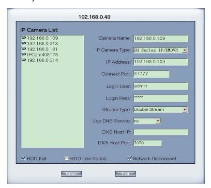
For example, when the redundant Hybrid-NDVR(192.168.0.43) happen some faults, such as Network Disconnect, HDD Fail and reboot abnormally. The IP Cameras of the associate Hybrid-NDVR(192.168.0.43) would add to the redundant Hybrid-NDVR(192.168.0.111) and all the added IP Cameras will Manual Record automatically.
