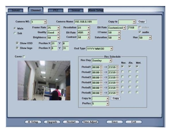
This section contains the parameters to designate a name for every camera connected, to enable or disable show LOGO and OSD, and to set display type of OSD & LOGO as well as record resolution, record type, record quality and frame rate, etc.
