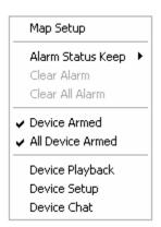
Click **Device Armed /All Devices Armed** (for more than one devices) to select alarm setup. Then, the device, including its cameras and sensors will turn golden yellow. When a camera detects a motion alarm, it will turn red and blink. At the same time, the video of the camera will be displayed automatically on the left screen if the setup in the server is suitable.
