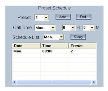
【Preset】It can add the preset into the Preset Schedule, the preset set completed in the Auto Pre yet, 【Call Time】【Schedule List】Set the time of the preset should be call at that time.
