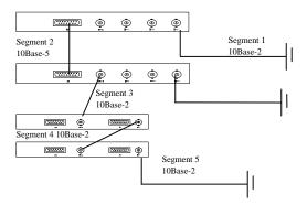
Note: Maximum 5 Segments (4 Repeaters) allowed. Each segment should terminated with a 50-ohm terminator in both ends.
