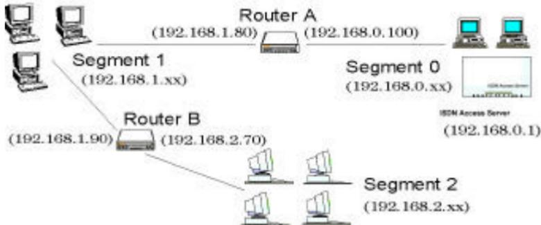
**Figure 21: Routing Example**
