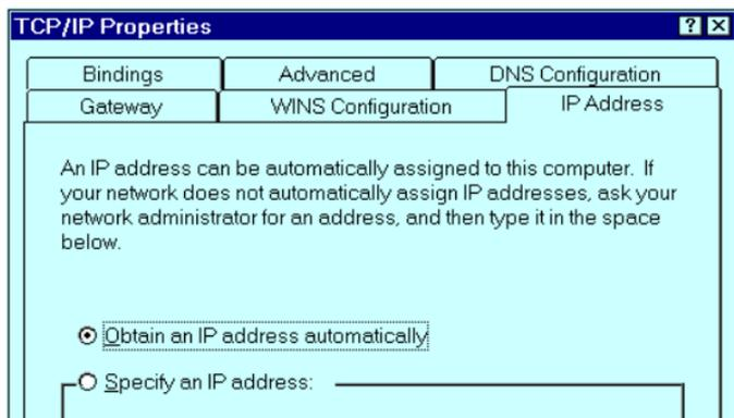
**Figure 7: TCP/IP Properties - DHCP**
