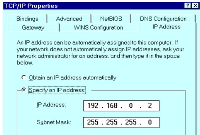
**Figure 8: TCP/IP Properties – Fixed IP Address**
