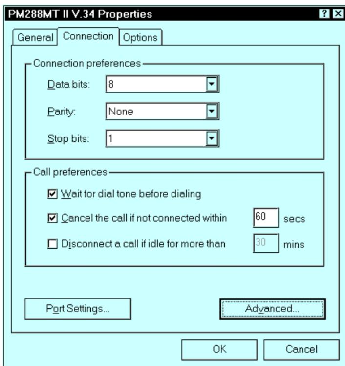
**Figure 28:- Connection Properties (W95)**
