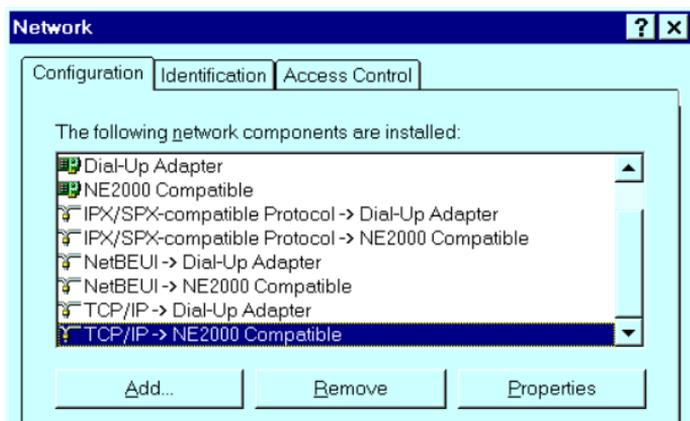
**Figure 6: Network Configuration tab**
