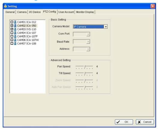
Install the PTZ camera following the instruction of the manufacturer. The PTZ camera is usually connected to the PC with RS-485.
