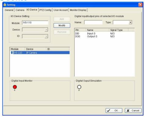
**Module Setting:** To name the module device and ID connecting the digital input/output device(s) to your system.
