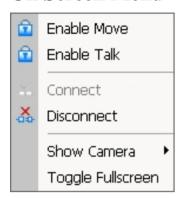
Right click on the camera screen and get the On Screen Menu from which you can **Enable Move**, **Enable Talk**, and **Connect / Disconnect** the camera.
