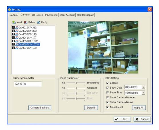
Camera List: The camera(s) connected to the system will show on the panel, click the name of the camera and then you may adjust the setting of it.
