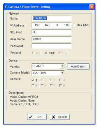
**Network:** Fill up the Network field (including Name, IP Address, Http Port, User Name, Password and Protocol) referring to the instruction provided by the manufacturer. Check "Use DNS" to use domain name instead of IP address.
