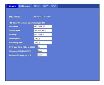
MAC address: Display the Ethernet MAC address of the device. Note that user cannot change it.
