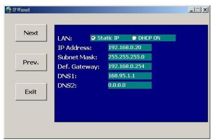
**LAN:** You can configure this ICA-310 to obtain its address automatically or manually assign. If there is a DHCP server in your network environment and you select "**DHCP ON**", ICA-310 can automatically obtain an IP address. If you don't have DHCP server or you want to use fixed IP address, please select "**Static IP**" and fill in the following fields with proper parameters.
