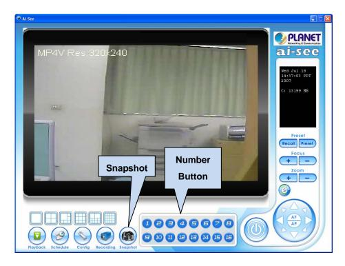
Please select the camera that you would like to capture with the camera number button. Then click the "Snapshot" on the main menu, click the "Snapshot" icon will capture a screen image and save the file into "Snapshot" folder. The captured file will be saved as JPEG format.
