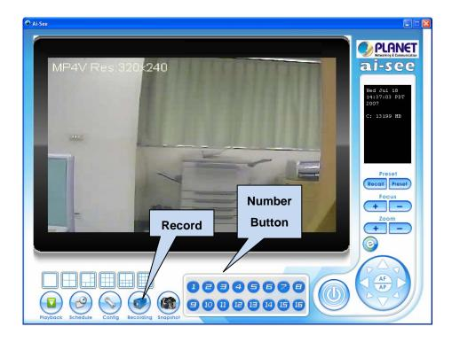
Please select the camera that you would like to record with the camera number button. Then click the "Record" on the main menu, click the "Recording" icon to start record video stream, press this button again will stop recording and save the record file into "Video" folder. The recorded video file will be segmented automatically per 5 minutes. Therefore, it will be 12 recorded files per hour. There will be a red spot on the window of recording camera to indicate this camera is recording.
