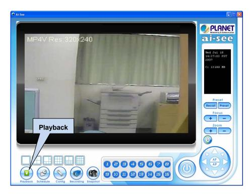
Click the "Playback" icon on main menu to playback the recorded video file. User should pick up a recorded file from recording video folder. Then the system will invoke system default media player to play the recorded file as below
