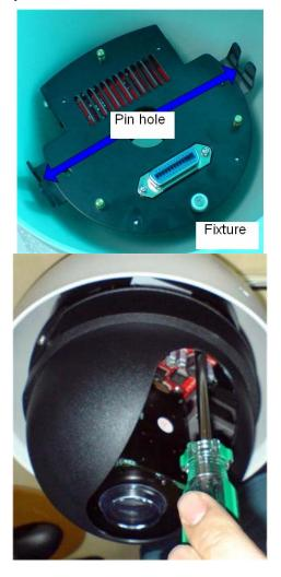
8. Follow anti-clockwise to fix the hemisphere cover onto speed dome.
