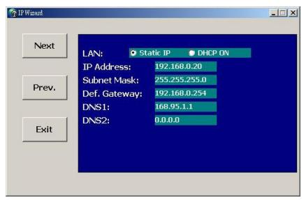
**LAN:** You can configure this ICA-601 / 651 to obtain its address automatically or manually assign. If there is a DHCP server in your network environment and you select "**DHCP ON**", ICA-601 / 651 can automatically obtain an IP address. If you don't have DHCP server or you want to use fixed IP address, please select "**Static IP**" and fill in the following fields with proper parameters.
