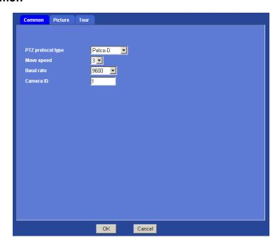
**PTZ protocol type:** The Network Camera is connected to built-in ICA-601 / ICA-651 and controls this device thru RS485 bus. It has three protocols that include Pelco-D, Pelco-P and K-ZM23S1N. Pelco-D is default protocol.
