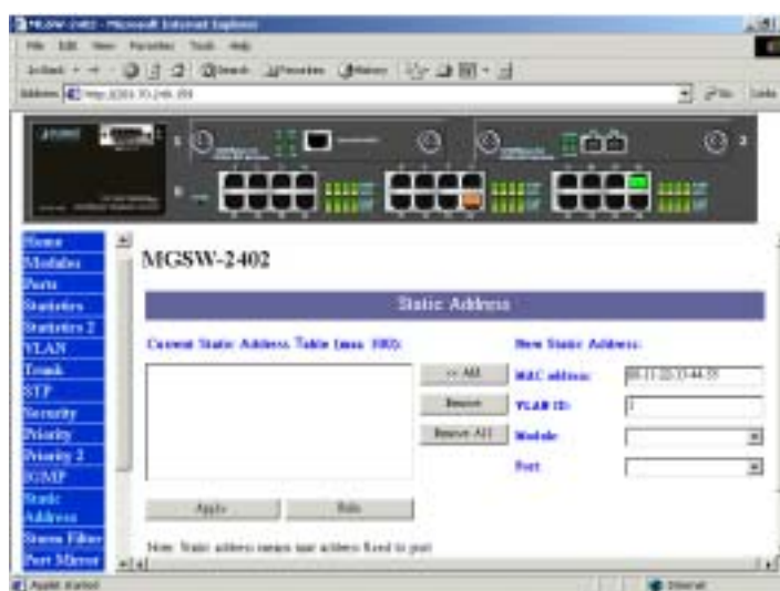
Figure 3-13 The Static Address page
