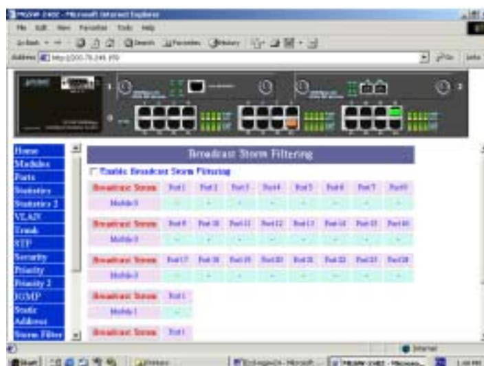
Figure 3-14 The Broadcast Storm Filter page
