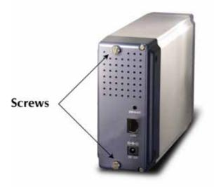
2. Grabbing the front panel and separate the HD holder from case.
