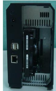
5. To install Disk 2 that located on right side (rear view), make sure HDD top face to right and connector side in front then slide the HDD into slot
