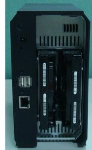
6. Put the rear cover of NAS-7200 back to finish HDD install
