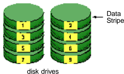
RAID 0 Striping interleaves data across multiple drives
