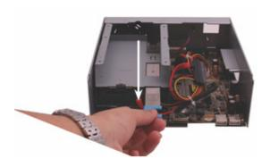
5. Place the hard drive into the tray and push it inward to secure the hard drive.
