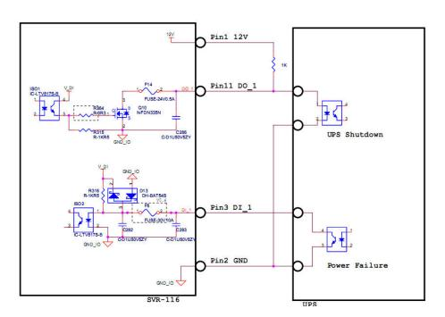
\* The NVR uses DI\_1 to receive signal from UPS system and uses DO\_1 to **shut it down.**
