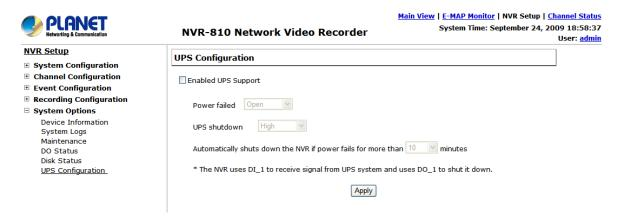
Connect UPS with its RS-232 interface to the NVR's 10 port:
