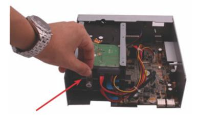
8. Place the top housing back and secure it with the bottom housing.
