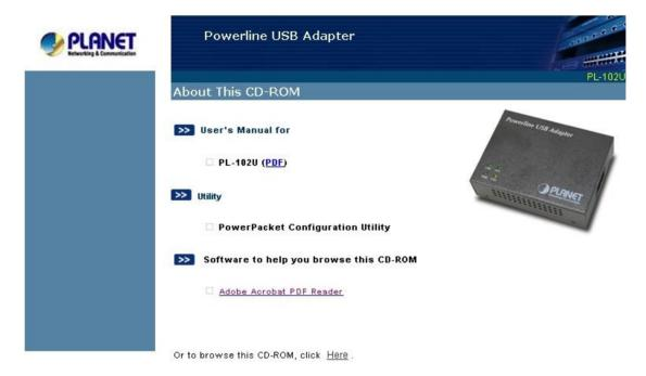
2. To install the utility, click on the "PowerPacket Configuration Utility" hyperlink to activate the installation procedure for the application program.
