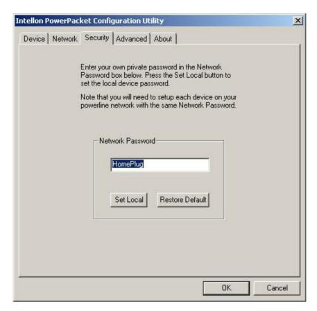
All PL-102U are shipped using "HomePlug" as a network password. The Security screen allows you to change this network password and set your own private password and apply it to PL-102U connected to the computer where the utility is running. Click Restore Default button to restore the original network password "HomePlug" and apply it locally. Click Set Local button to change the network password locally.
