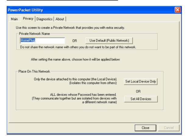
The **Privacy** tab will allow you to change the **Network Password** to the unit that is currently connected to this computer. This network password encrypts all data that is sent from this unit using 56-bit data encryption standard (DES).
