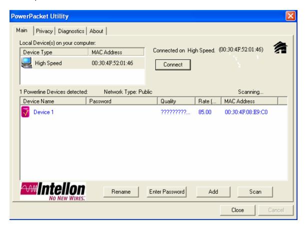
The Main tab shows the powerline units that are connected to the current computer and other powerline devices on the home network, and It will also display Mac Address of each device.
